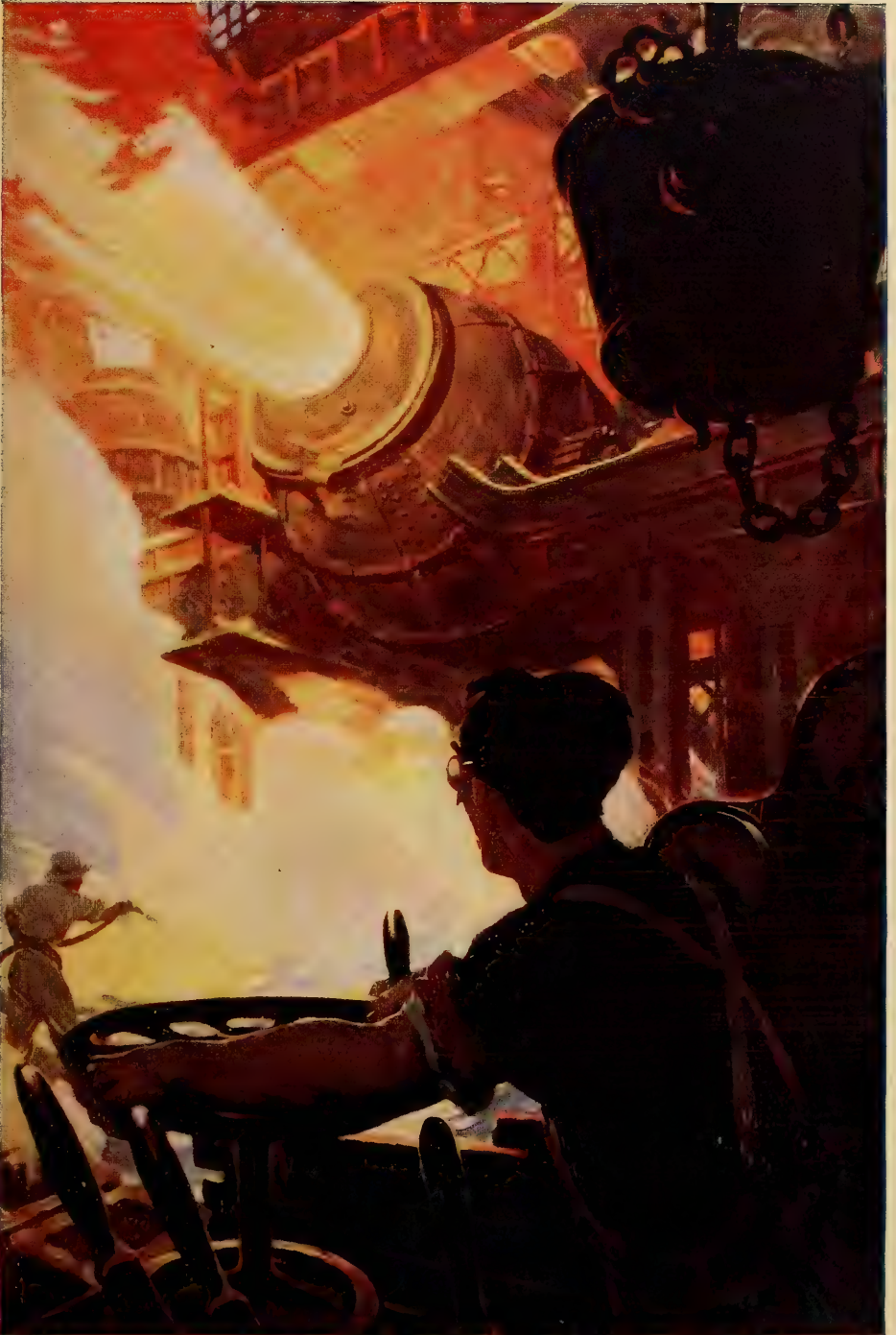
FROM IRON TO STEEL—The Bessemer Converter blasting the impurities from the molten iron.
